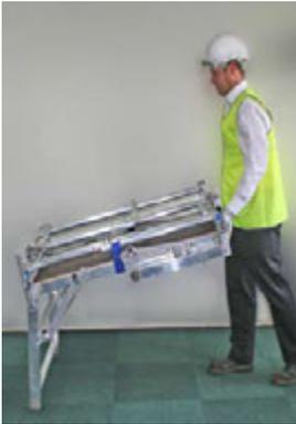
It is possible to wheel the unit into the precise job location when first leg assembly is complete.
