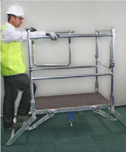
When accessing platform, keep body's centre of gravity towards platform.
