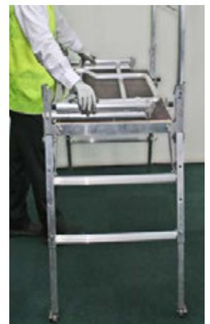
Disengage base of guardrail and lay guardrail unit onto platform.
