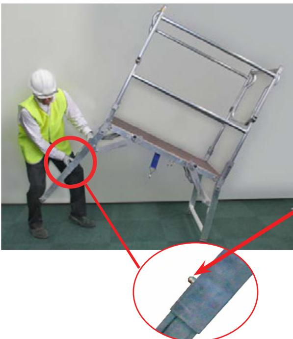
The platform height is also adjustable by extending the telescopic leg (3 positions).
