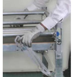
Lift one end of platform and simultaneously pull the leg assembly out until legs automatically lock in place.
