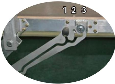
There are 3 positions in which the lever can be placed.
