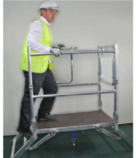
Once access has been gained, immediately close guardrail behind you to provide protection to all 4 elevations of platform.
